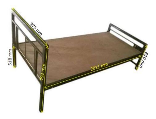
Iron Cot :  $6\frac{1}{4}$ ' X 3'; 16 Guage Square pipe; Four bottom supports with 18mm plywood; chemical treatment; red oxide spray with powder coating finish; Nickel Gray colour & pvc bushes at the bottom
